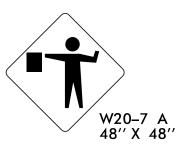
PLACED 500' IN ADVANCE OF FLAGGER. PLACED 250' IN ADVANCE OF FLAGGER.
